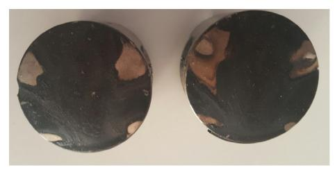
See pic on the Left for a set of pistons showing good piston wash, Piston wash (clear areas on a pistons surface) is created by the incoming unburnt fuel mixture cooling the piston surface as it enters via the transfer ports. The carbon deposits are only burnt on to the top of a piston where it is the
