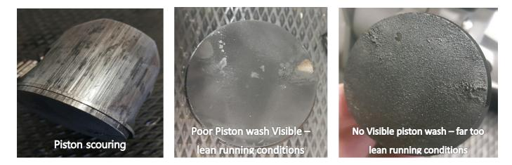
The second feature noticeable on a lean run is the underside of the piston surface (Remember "Black Spot Hot" – see pics below) when the piston temp is higher than it should be, the unburnt fuel from the crankcase will actually also burn a black spot onto the underside of the piston.
